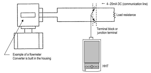
Figure 11.1 Connections to the Current Output Line
